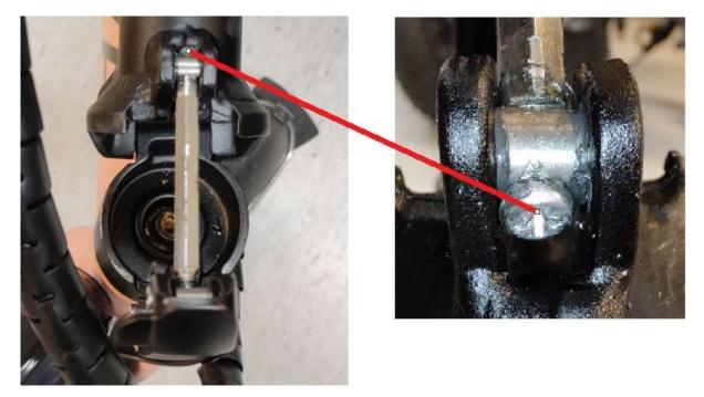
Now you can adjust the metal pin. To tighten turn with the clock. To loosen turn anticlockwise.
