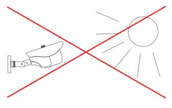
It is possible to adjust the cap of the camera. If you get distorted colours or glare then try and adjust the cap of the camera, as this will help in many situations.
